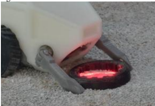
Figure 3: The robotic elements to place the electrodes on the surface are the only moving elements in the mining collection system
